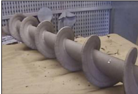
Worn screw after first weld overlay and grit blasted ready for coating
