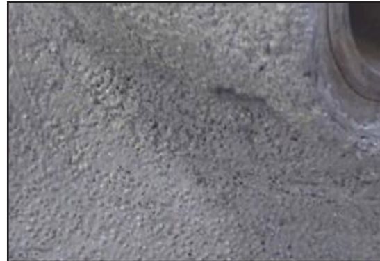
ARC BX1* is applied as severe duty wearing coat
